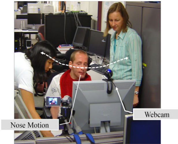
Fig. 1. A user conducted an experiment where he moved his head left and right. The exaggerated white line indicates the motion of his nose feature.
